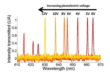
Fig. 1 Filter transmission showing wide range single mode tunability. The transmission lines indicated are  $TEM_{00}$  modes (see text). The weaker transmission lines below 625 nm are  $TEM_{01}$  modes.
